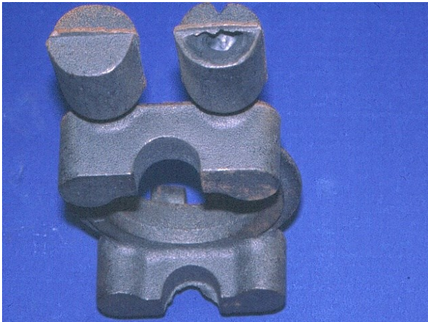
Figure 13. Bracket casting with 2 top feeders: Only 1 feeder has piped.
