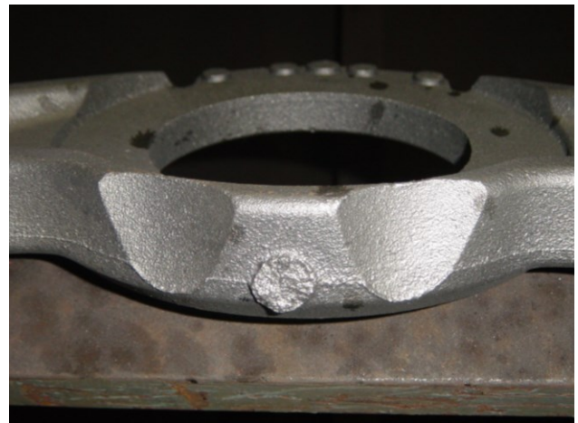
Figure 11. Photo of the contact area with a single feeder.
