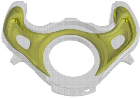
Figure 8. Plot of transfer modulus of 0.645 cm in the casting.
