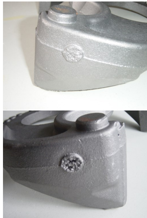
Figure 4. Feeder contacts with original design (2 feeders).
