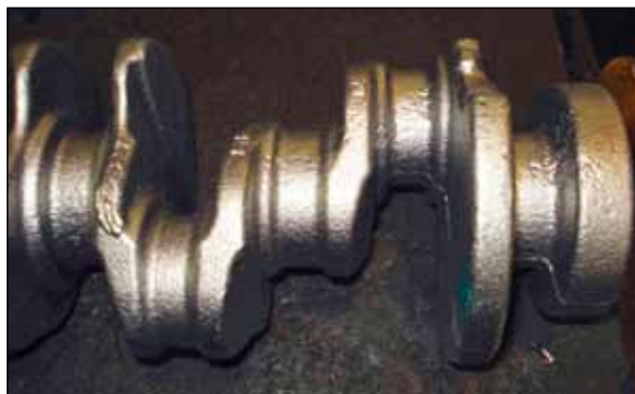
Fig. 3. The surface imperfections in this crankshaft are aligned to the flow path from right to left due to excessive metal speed at the riser gate.
