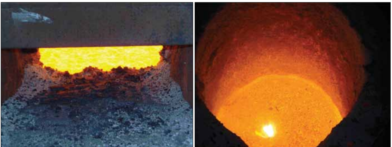
Fig. 6. At left, fluid slag is shown on the melting furnace at 1,480C before treatment. At right, the same melt is shown after treatment with high magnesium (80%) cored wire.
