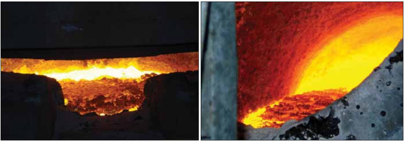
Fig. 7. At left, high melting point slag is shown before treatment after addition of 0.5% of silica sand. Even if the tapping temperature was similar, the liquid iron appears brighter than in Fig.9a. At right, the same melt is shown just after treatment with high magnesium (80%) cored wire.
