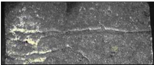
Fig. 4. Shown are false cold laps due to further iron oxide enrichment as a consequence of surface oxidation
